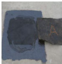
Successful peel test example
